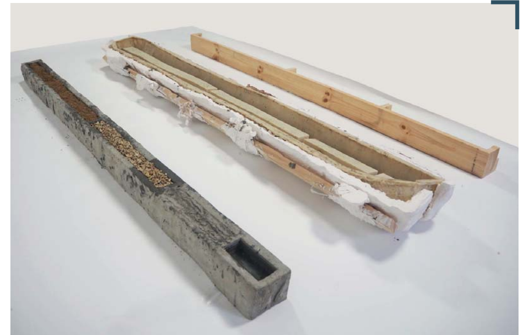
A model that highlights the process of production. The concrete model is divided into the material ratios to produce concrete and the components are measured to equal the volume of the outer concrete structure. Materials: Water, cement, aggregate, sand, concrete, plaster, vinamould, wood.
