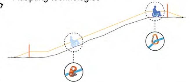
Combining the adapted technologies and rope/cable systems allows for a simple safety system permitting the wheelchair athlete to scale inclines without the anxiety of falling backwards.
