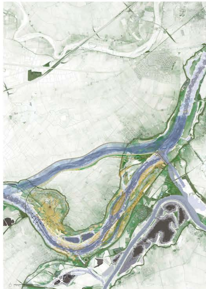
2. Demonstration Bend of Sint Andries; from clogging channels to two types of waterways. A navigation channel. A waterway without ships but with lots of fluctuation in water levels and sedimentation.
