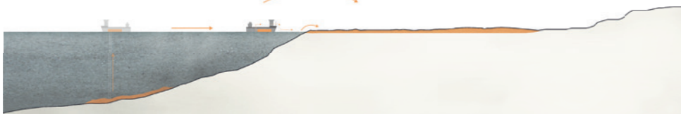
production of the sand engine
