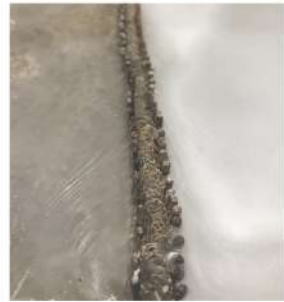
Detail model: double raw of wooden poles filled with branches lets the water pass and traps the sediments. Opposite to a normal groyne, its permeability allows for uniformity of sedimentation.
