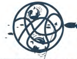
ATTACHING NATURAL OR SYNTHETIC FIBERS TO THE REEF MODULES CAN BE BENEFICIAL. THEY MAKE A VERY ATTRACTIVE SUBSTRATE FOR THE SMALLEST OF CREATURES AND ARE IDEAL PLACES FOR CUTTLEFISH TO LAY THEIR EGGS.
