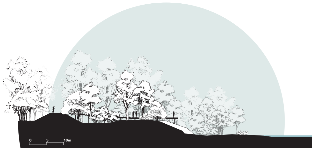
Detail section of new accesses to the river through the construction of new platforms crossing the riparian zone.
