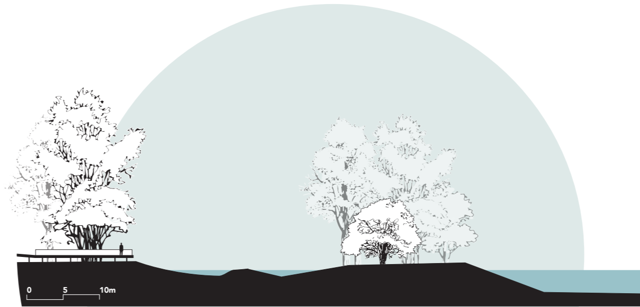
Detail section of the river requalification operation with the creation of secondary channels to widen the river section and the creation of new ecosystems.
