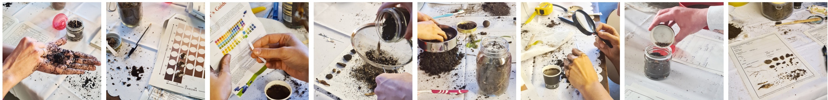
▲ The analysis sequence carried out during the workshop, which included an examination of grain size, texture, colour, pH level, temperature, moisture content and material composition.
